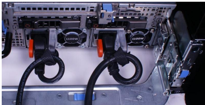
Figure 2. Routing power cables through the strain reliefs
